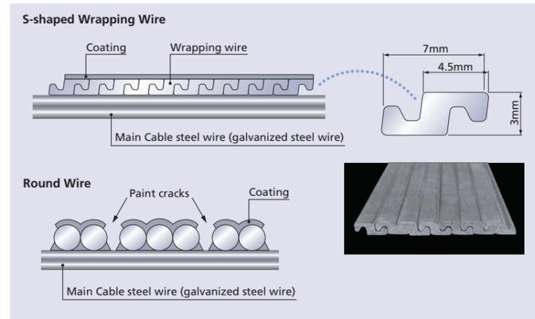
This S-shaped wrapping wire prevents cracking of coating by mean of the effect of interlocking of turns. The adoption of coating agent having an excellent elongation performance prevents from cracking due to expansion of cables and at the same time prevents the infiltration of rain water and others.
