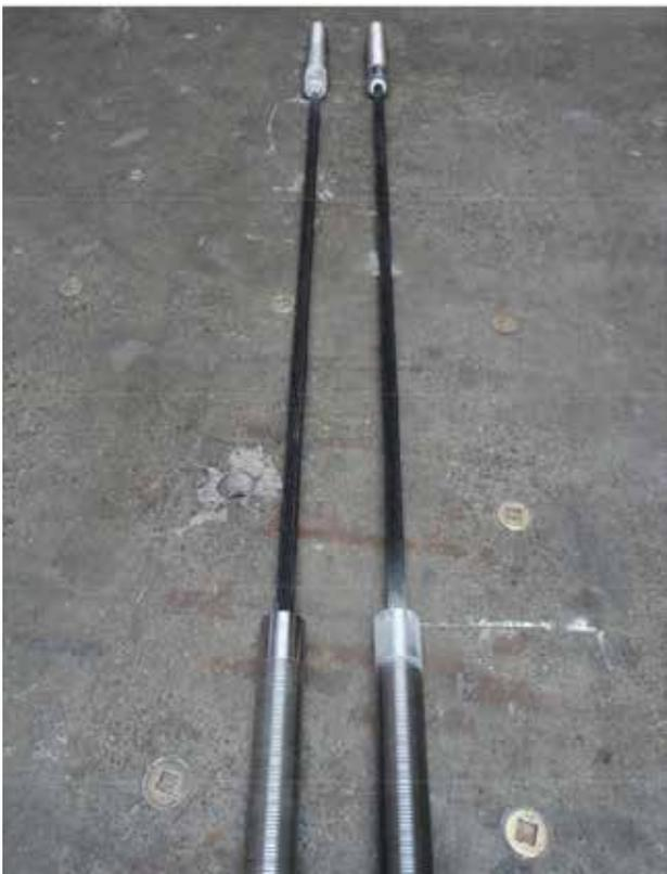
CFCC strands with pre-installed anchoring devices
