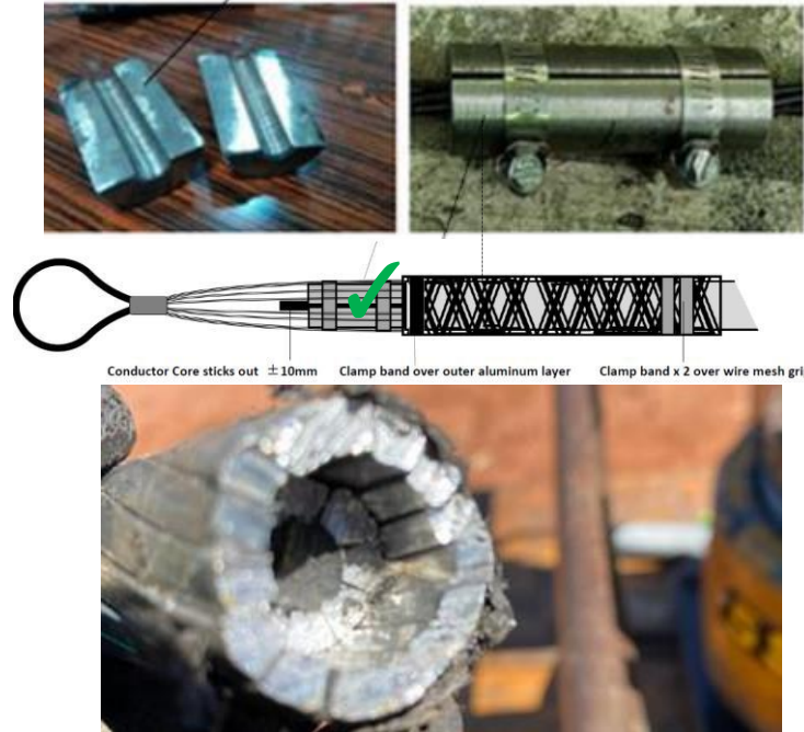
CFCC core can slip inside aluminum layer by tension stringing
