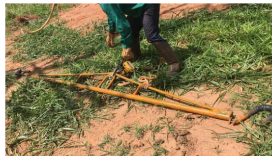
Triangle frame hoist for lifting conductor for suspension clamp
